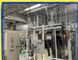
GaN crystal growth equipment for high-temperature and high-pressure condition
