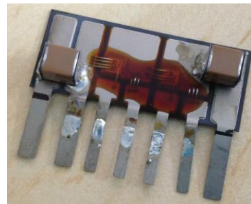
Low inductance package for SiC power module
