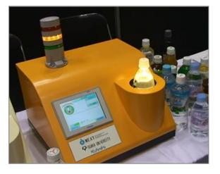
We developed the liquid explosive detection technology using NIR with the aim of inspecting liquids, such as drinking water, before they were brought on board an airplane. We changed the density of hydrogen peroxide and measured the NIR spectrum. The NIR spectrum provided adequate detection of hydrogen peroxide water in the PET bottle.
