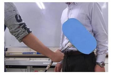
Some individuals may attempt to bring unauthorized or explosive chemicals to an airplane by hiding them in clothes or luggage. We developed the NQR inspection equipment to detect explosive and unauthorized drugs. The NQR is a new sensing technology that relies on the specific resonant frequency which occurs to the atomic nucleus when it is irradiated.
