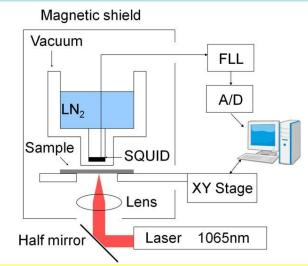
We have performed the non-contact inspection of the semiconductor with the laser SQUID microscope. The photo-excited current flows when the semiconductor is irradiated with light of greater energy than that of the band gap energy. We measured the magnetic field distribution generated by this current, and investigated the defect area of the sample.
