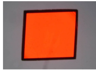
DAST single crystal ( 3.0 \times 2.5 \times 0.362 \text{mm}^3 )
